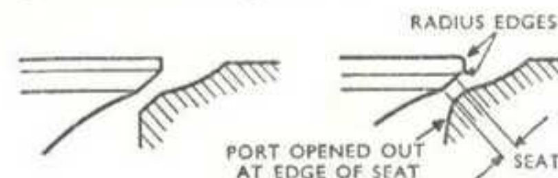
How to reduce the width of the seatings on valve face and inlet port.
